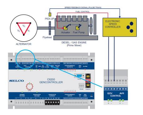
C6200 FlexGen controlling electronic speed governor by a DC voltage.
