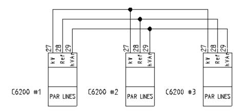
Please note that terminal 28 (COM) is internally connected to terminal 32 (Supply minus). In rare situations "gound loops" can cause noise to be injected into the application. Ground loops happen when multiple COM connections between modules (e.g. parallel operating C6200 units) exist. Ground loops can be avoid by only using terminal 32 as the common connection point for all COM connections.
