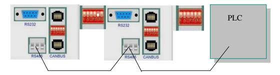
It is sometimes necessary to fix the potential of the RS485 + and – lines due to interference from other sources. This is done with two 1 k $\Omega$  resistors using a technique called "Biasing". One resistor is fixed between RS485 B and an external +5 V DC supply, the other is fixed between RS485 A and the reference of the -5 V DC supply. The reference of the 24 VDC (terminal 32) supply must then be connected to rightmost terminal of the RS485 plug on each and every module.
