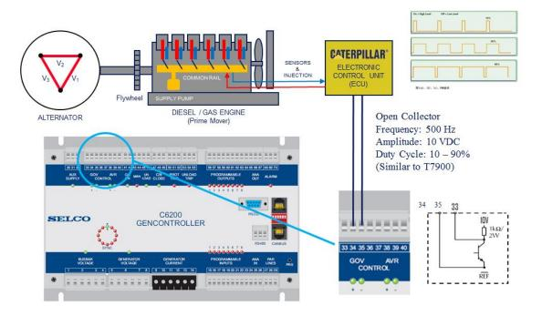
C6200 FlexGen controlling ECU by a PWM signal.
