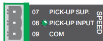
The pick-up LED is on when a pick-up signal is received (engine turning), off when the engine is stopped and flashing when the connection to the pick-up is lost (frequency 1,25Hz, duty cycle 10%).
