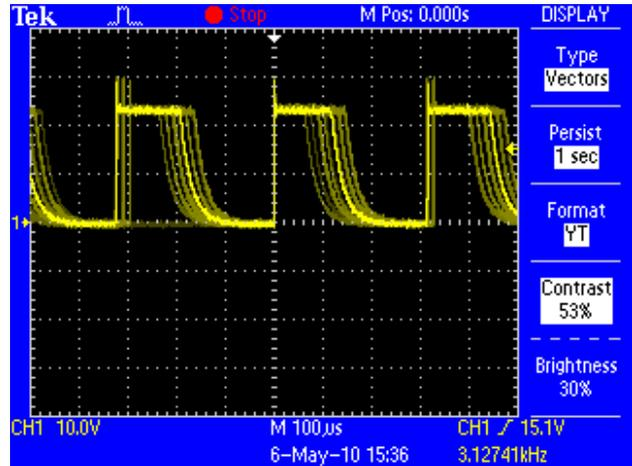
As can be seen on the right hand picture, it is important to trigger the pick-up input from the correct flank. For the PNP pick-up this is the raising flank.
