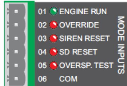
A LED is dedicated to each input. The LED is lit when the input is active, off when the input is inactive.
