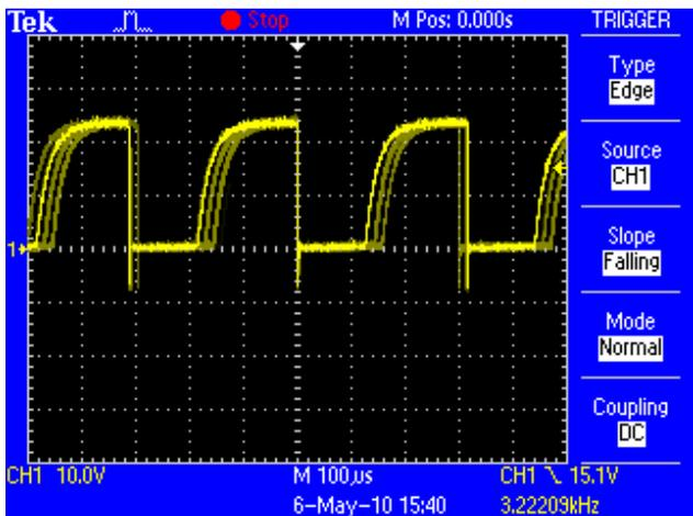
As can be seen on the right hand picture, it is important to trigger the pick-up input from the correct flank. For the NPN pick-up this is the falling flank.
