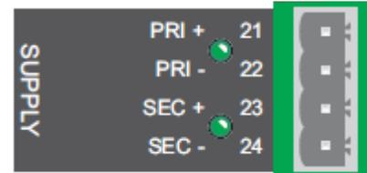
In case any power supply fails an alarm will be generated on the common alarm output and the siren relay will be de-energized (normally energized). Power supply failure alarm disappears automatically when the power supply returns.
