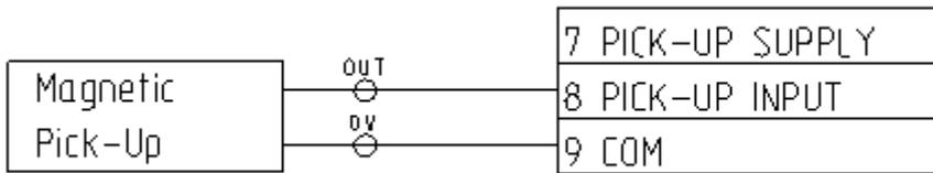
The minimum Voltage from the pick-up is  $U_{min}$ , pk-pk = 6V
