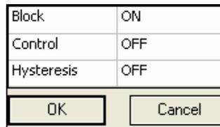
There are three “flags” which can be set ON or OFF using the “Flags” parameter in the alarm section. The “Block” flag represents the status of the alarm blocking function. The related alarm will be blocked by the first block control input when it is set to “ON”. Input terminal 1 of group 8 is the first block control input as described above.
