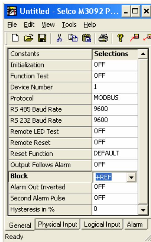
Selecting “+REF” or “-REF” will make the alarm block function available. Selecting “+REF” will cause all alarms with a “Block” flag to be blocked, when input 1 of group 8 (IN81) is connected to + of the supply voltage. Selecting “-REF” will cause alarms with a blocking flag to be blocked, when input 1 of group 8 (IN81) is connected to GND.
