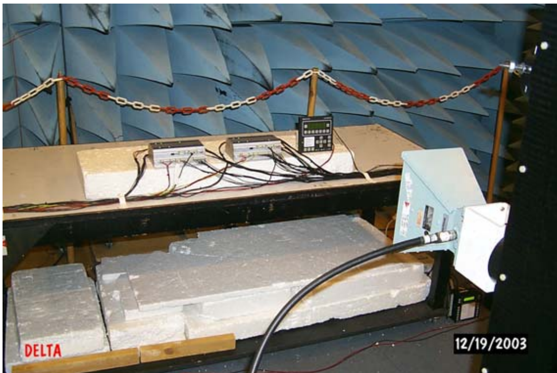
PHOTO 16. Radiated radio frequency interference (1000-2000 MHz).
