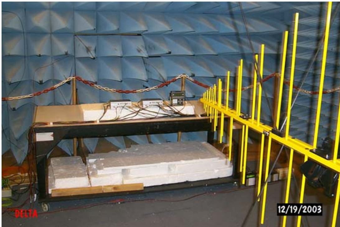
PHOTO 15. Radiated radio frequency interference (80-1000 MHz).
