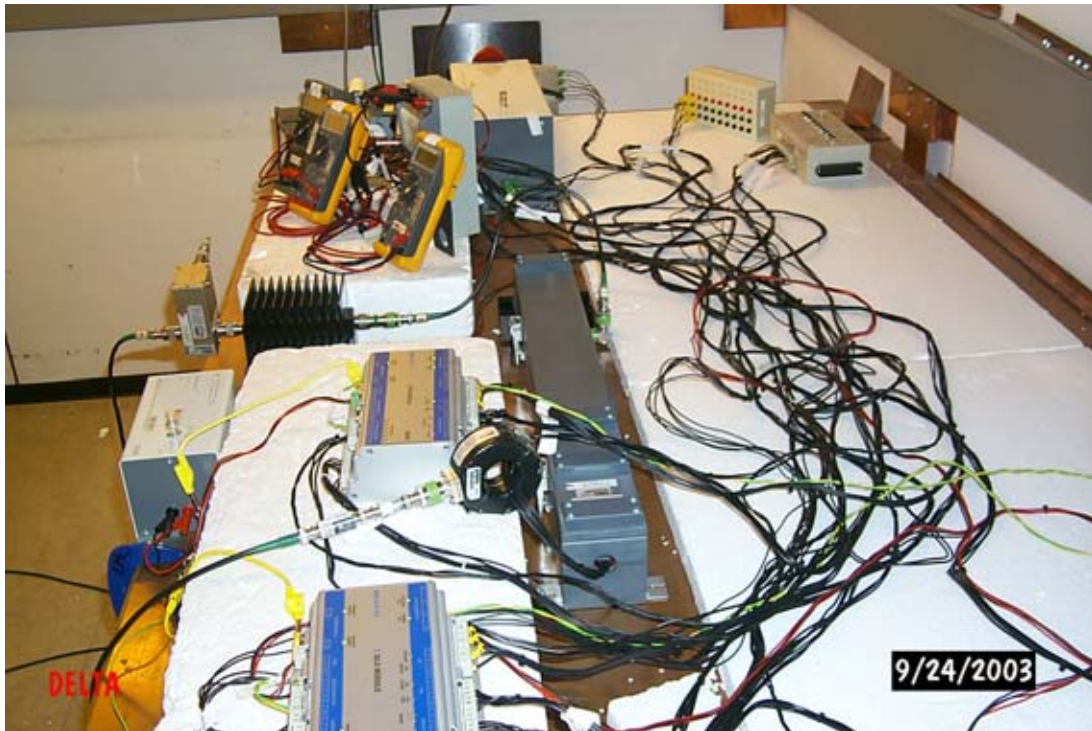
PHOTO 3. Conducted radio frequency interference.
