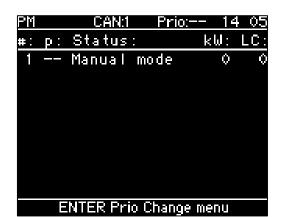
Above display shows that the generator has no assigned priority (--) and is in manual mode.
