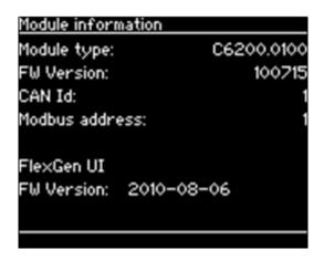
Module Type: Type of connected generator controller (here C6200.0100)
