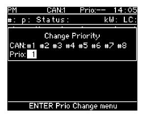
Above display indicates that the connected C6200 has CAN address 1. The Priority of the generator is 1 (first to start). Use the cursor up/ down keys to change priority. Press [ENTER] to accept the change. The display will move back to the PM menu.
