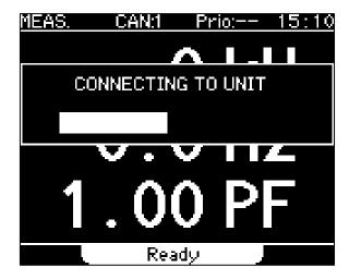
After communication has been established C6500 moves to the measurement (MEAS) display and shows measurements.
