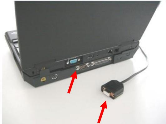
Connect the DB9 female plug of the communication cable to the male DB9 RS232 port of the PC.
