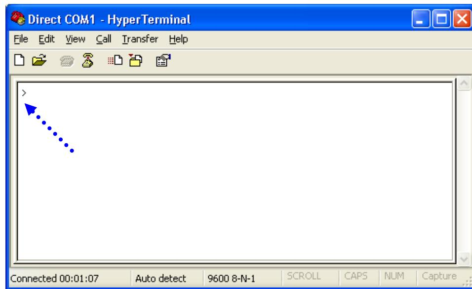
Hit the *ENTER* key to check the connection to the unit. Provided that the connection is OK, the SELCO G-Line relay or T7900 should respond with a ">" prompt. This means that the relay is ready for communication.
