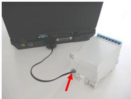
Connect the RJ11 modular plug of the cable to the PROG connection located at the rear side of the SELCO G-Line relay or the front of T7900. You will need to depress the small plastic tab in order to make the plug “snap” into the connector.
