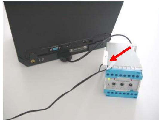
Connect a +24 VDC power supply to the SELCO G-Line relay or T7900. The positive wire (+) connects to terminal 9 and the negative wire (-) connect to terminal 10 of the G-Line relay (terminals 11 and 12 respectively of the T7900). Turn on the power supply and check that the green PWR LED ignites.
