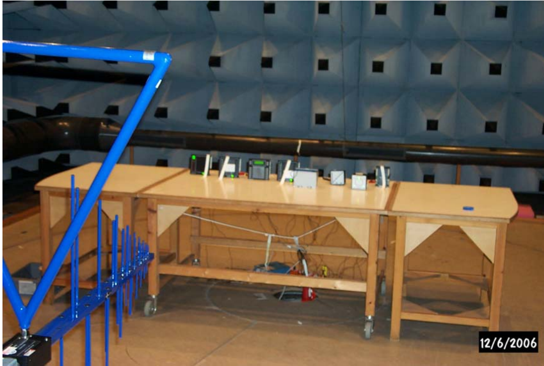
Photo 1. Radiated emissions (1000 - 2000 MHz)
