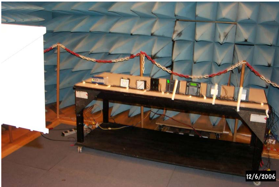
Photo 2. Radiated radio frequency interference (1000-2000 MHz)
