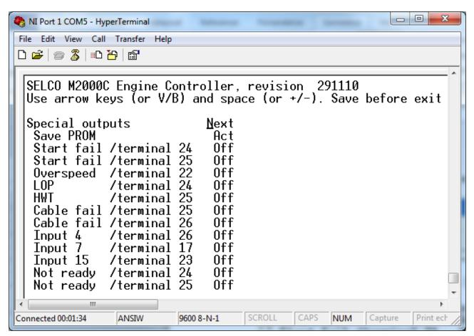
When activated in the configuration the cable fail output will activate in case a cable fault on any of the sensor outputs is detected. In case another cable fault appears while the output is already active, the output will deactivate for 2s and then activate again.
