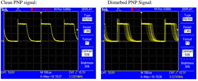
As can be seen on the right hand picture, it is important to trigger the pick-up input from the correct flank. For the PNP pick-up this is the raising flank.
