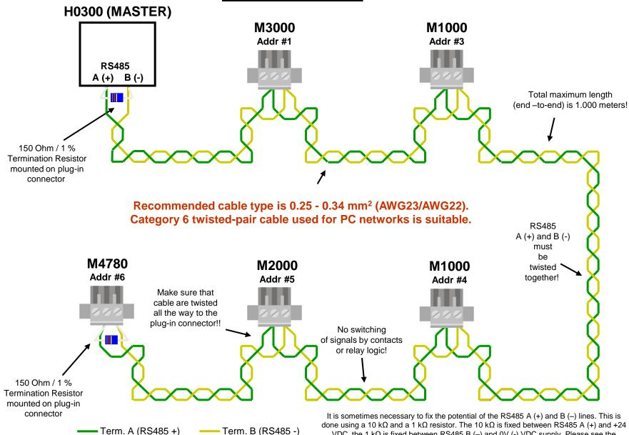
VDC, the 1 k $\Omega$  is fixed between RS485 B (–) and 0V (-) VDC supply. Please see the MODBUS biasing document in the alarm panel document section.
