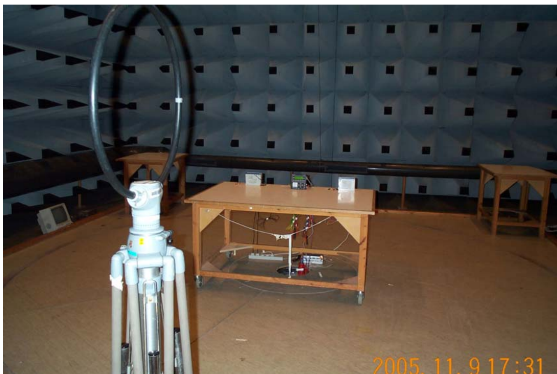
Photo 8. Radiated emissions (0.15 - 30 MHz). 3 m.
