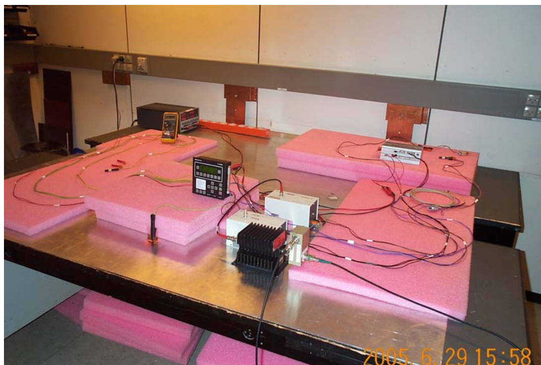
Photo 11. Conducted radio frequency interference, e.g. S6610.
