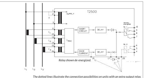
The dotted lines illustrate the connection possibilities on units with an extra output relay.
